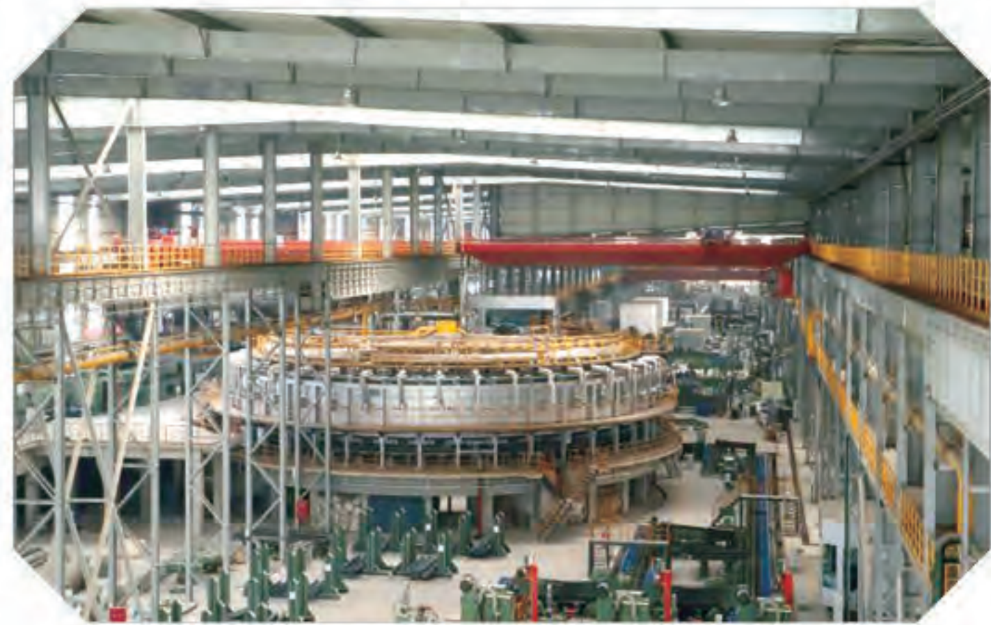
25 米环形加热炉 25m Rotary heating furnace
