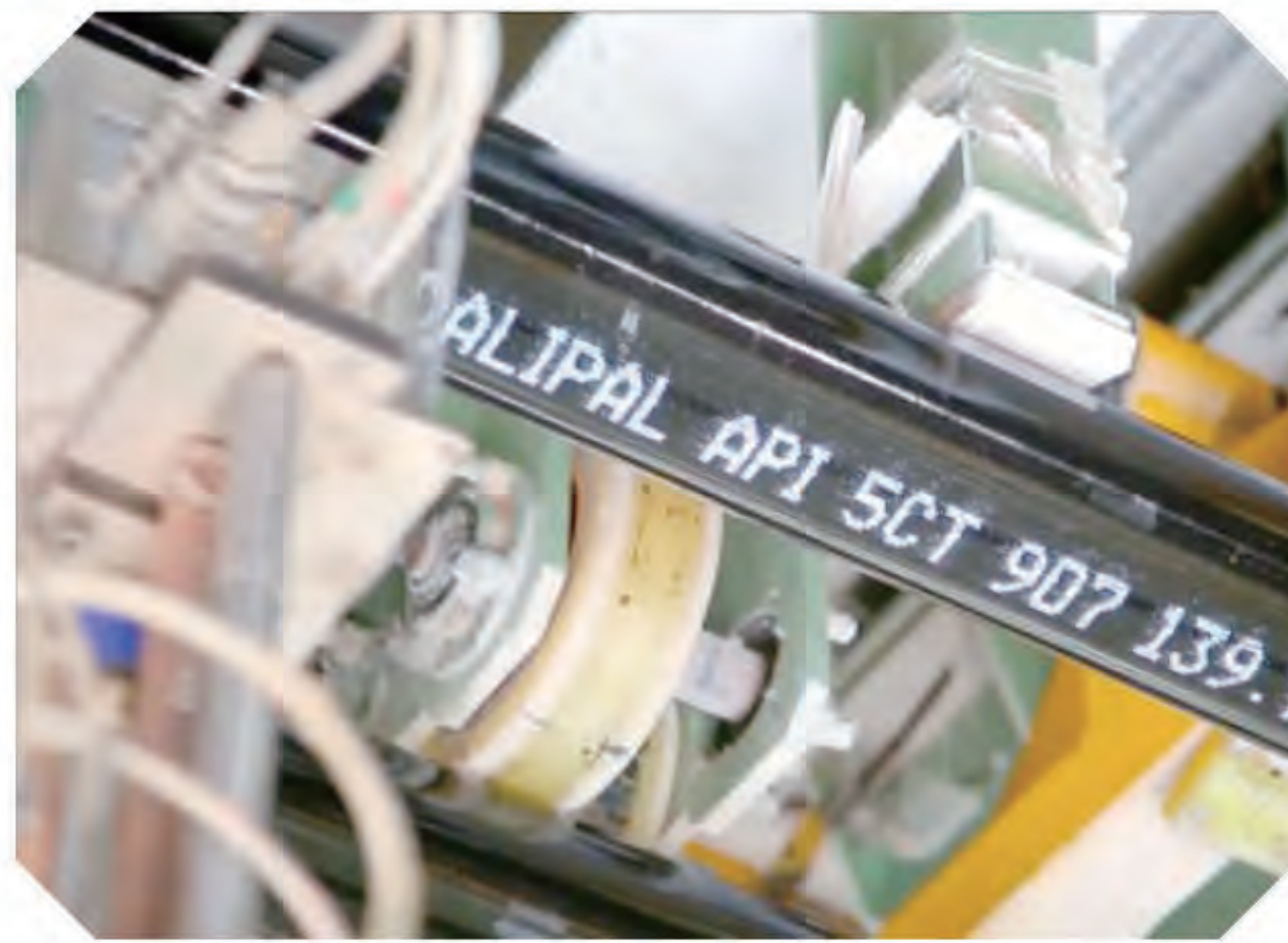
测长、称重、喷标设备 Length measuring, weighing, and code spraying equipment
